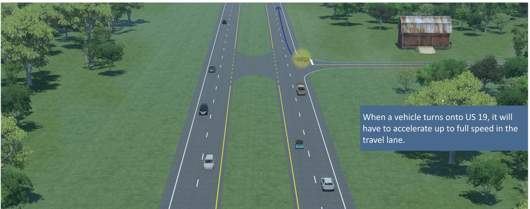
When a vehicle turns onto US 19, it will have to accelerate up to full speed in the travel lane.
