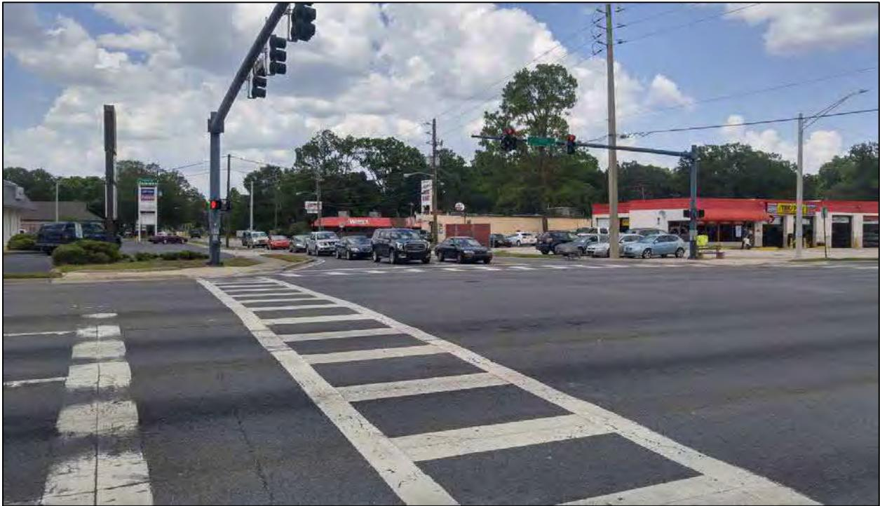
**Photo 9: Looking north: Note faded stop bar on the west leg**
