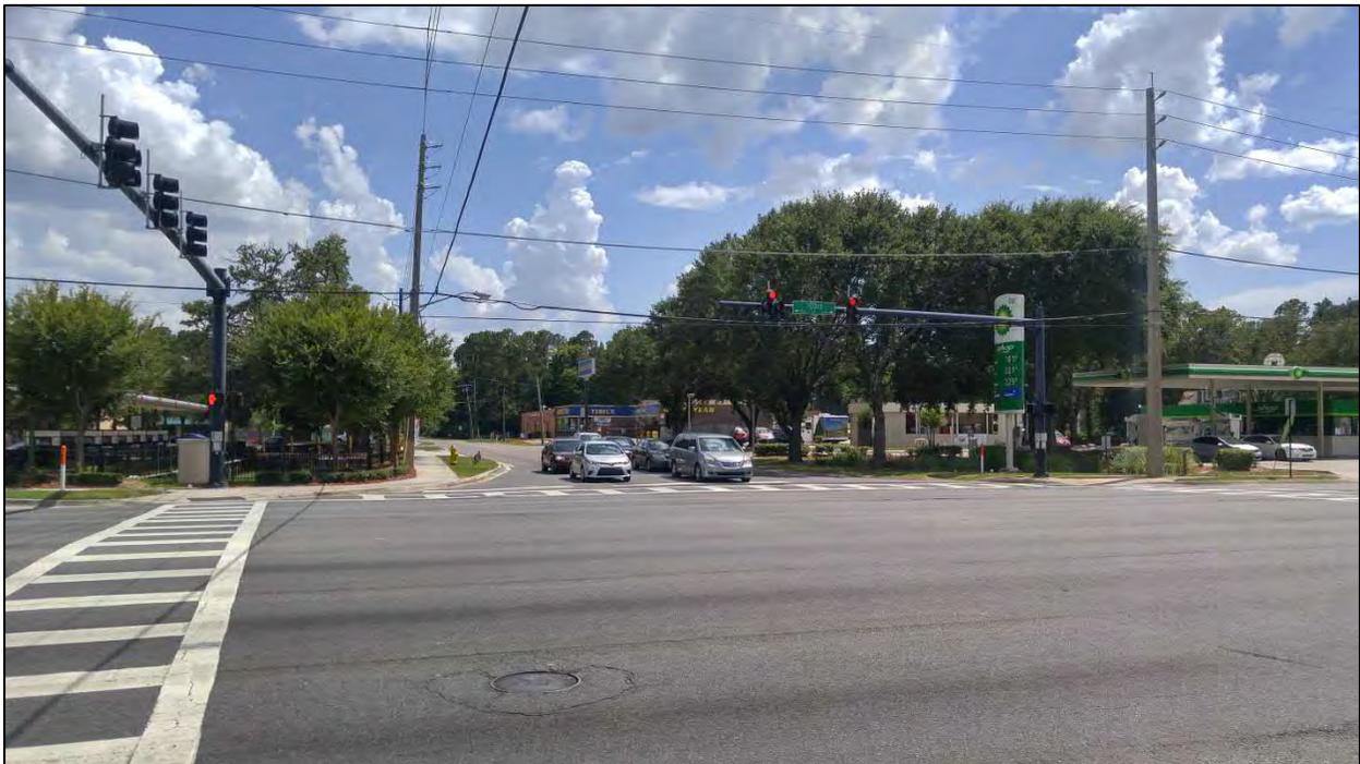
**Photo 6: Looking south: Note pavement rutting and cracking within the intersection**
